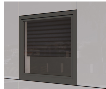
Version 2 flush with the facade
